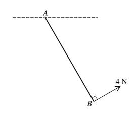
A uniform rod AB of weight 16 N is freely hinged at A to a fixed point. A force of magnitude 4 N acting perpendicular to the rod is applied at B (see diagram). Given that the rod is in equilibrium,
